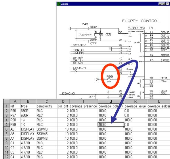
In the example shown, resistor R99 has been highlighted within the schematic viewer and allocated the following PPVS coverage values: Component **[P]**resence = 100%; Component **[P]**olarity = 100%; Component **[V]**alue = 0.0% and Component **[S]**older = 100%
