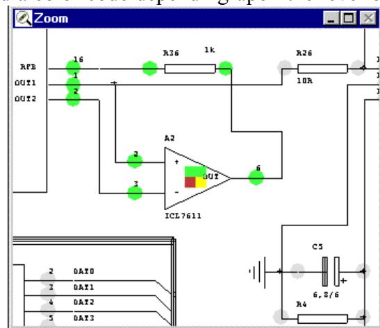
Initially, all selected devices inherit 100% coverage for each of the Presence, Polarity and Value facets. The coverage figure could be graphically updated to reflect customer estimation. The Solder coverage is computed, based on the number of covered pins divided by the total number of device pins.
