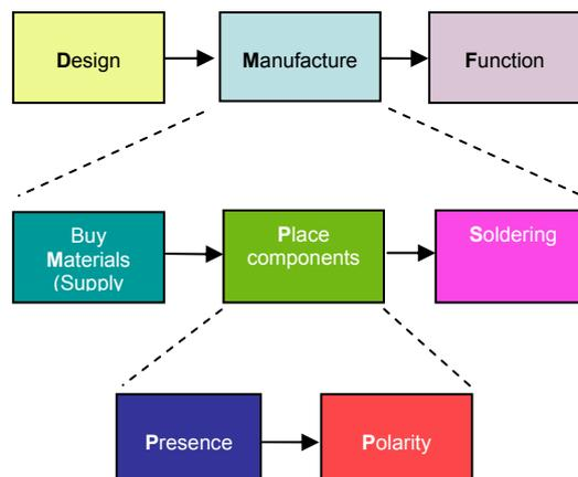
If we now take these additional defect classes into account, the test coverage model now becomes **DMPSF**: **D**esign, **M**aterial, **P**lacement, **S**older and **F**unction.
